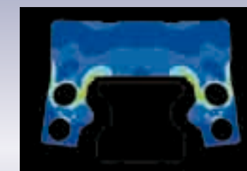
Example of roller slide deformation analysis
